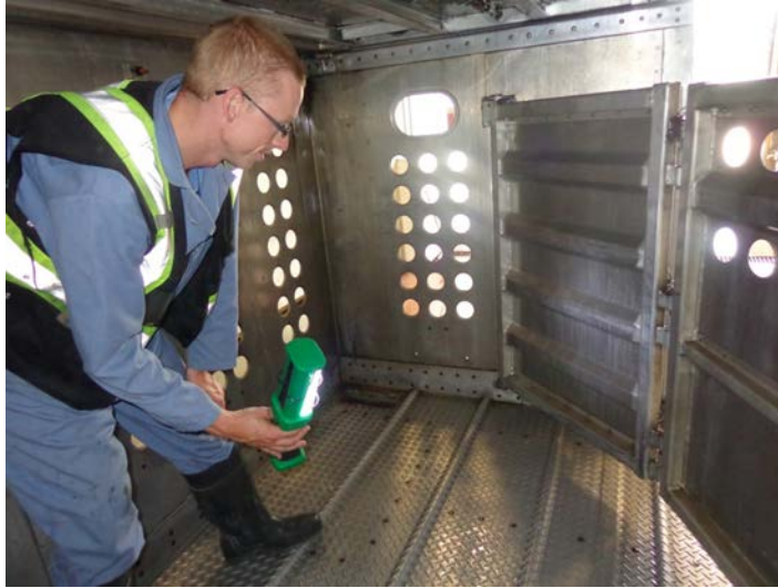
Figure 10: When inspecting a transport unit for the presence of organic matter, use a light to inspect a low-lit areas and move gates or doors so that all areas are visible, as illustrated in this livestock transportation unit.
