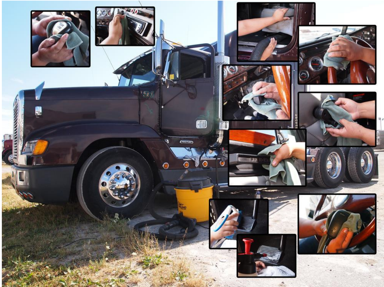
Figure 12: Illustration of common contact areas in the power unit that require additional attention when cleaning and disinfecting. Photo credit: Ontario Swine Health Board Truck Wash Handbook.
