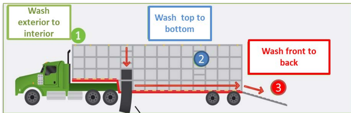
Figure 8: When rinsing the transport unit, avoid re-introducing organic matter from areas that have already been rinsed by starting with the exterior (1), then the interior (2) and working spraying from top to bottom and front to back (3). Modified from the manual entitled " Live Hog Transport Vehicle Wash/Disinfect/Dry Protocols " by the Canadian Swine Health Board 2011.
