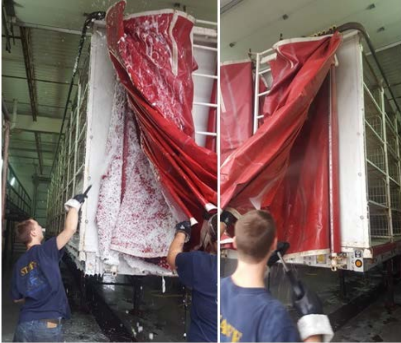
Figure 9: When washing, apply detergent to all surface areas (left) working from the bottom towards the top, as illustrated in this poultry trailer. Rinse the detergent or degreaser and any organic matter working from the top down. Repeat the washing step until all organic matter has been removed.
